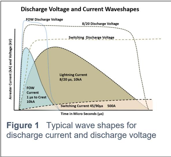
**Figure 1** Typical wave shapes for discharge current and discharge voltage
