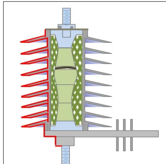
**Figure 4** Demonstration of creepage distance
