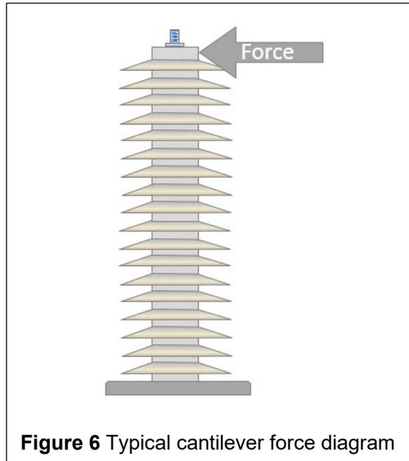
**Figure 6** Typical cantilever force diagram
