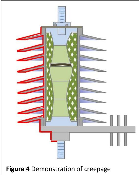
Figure 4 Demonstration of creepage
