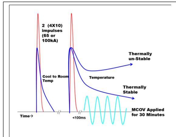
**Figure 2** High-current, short-duration energy withstand test
