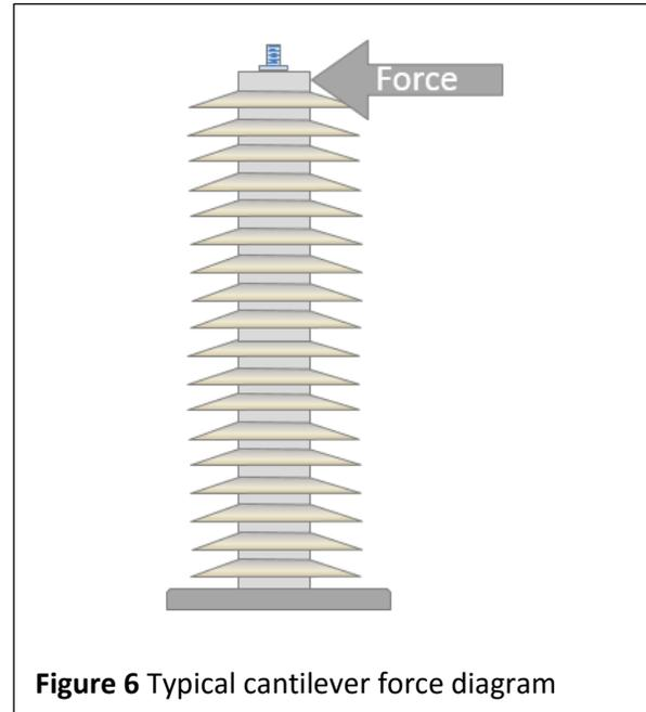
**Figure 6** Typical cantilever force diagram
