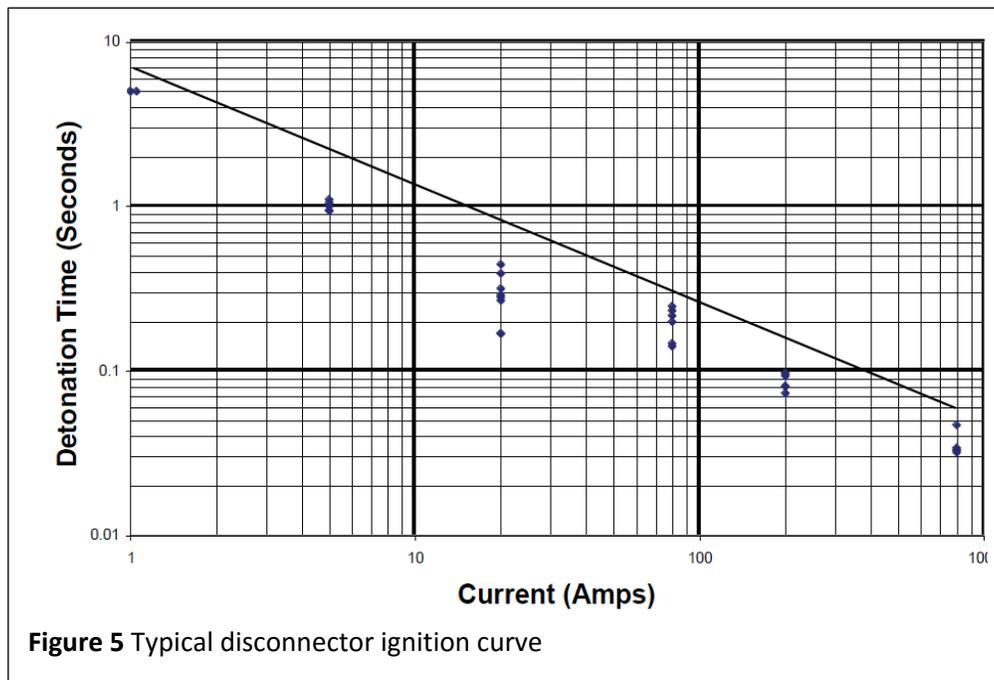
Figure 5 Typical disconnector ignition curve
