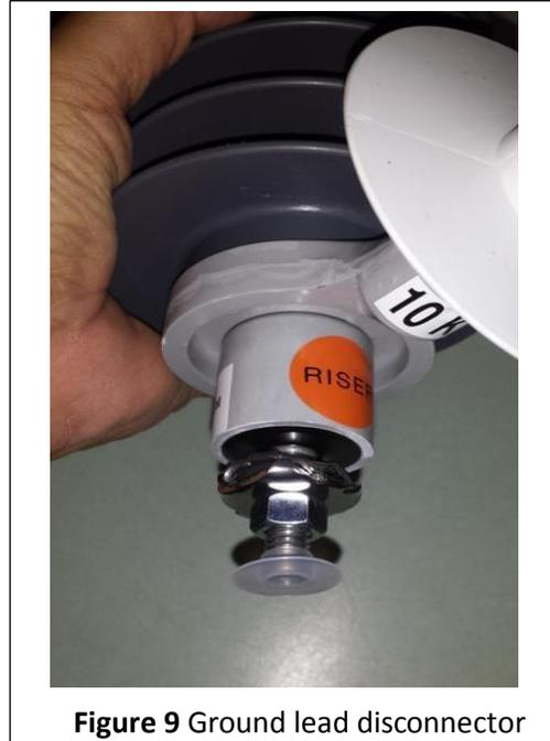
**Figure 9** Ground lead disconnector
