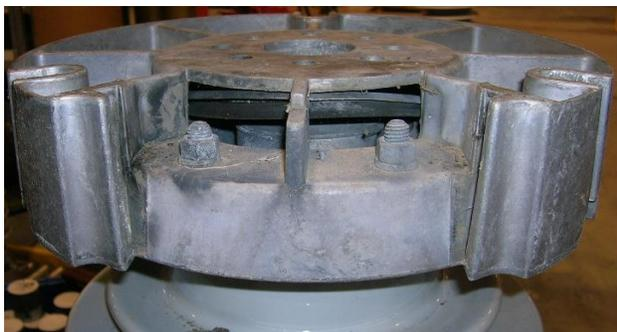
**Figure 11** Top vent of a 60kV porcelain-housed arrester that has successfully vented as designed
