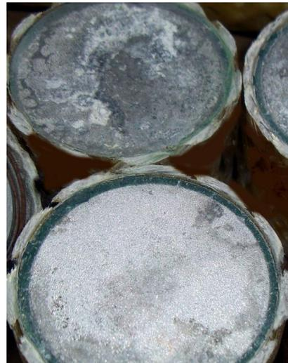
**Figure 6** A polymer-housed arrester with poor moisture ingress design resulted in this internal corrosion and premature failure
