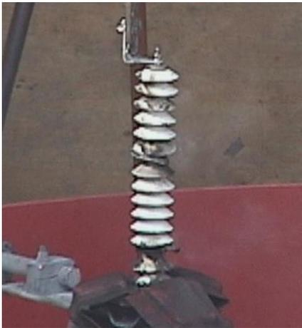
**Figure 7** Transmission line arrester after short-circuit test
