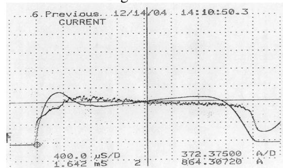
The measured energy integration for the gapped SiC design will vary from discharge to discharge depending upon the consistency of the current limiting performed by the gaps. Both of the above examples were simulations of the typical performance of each type of arrester when applied to a 345 kV system. The line impedance, charge, and length characteristics were specified in Table 4 of IEEE C62.11.
