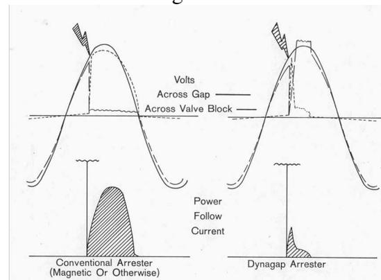
Implementation of the current limiting gap significantly reduced the energy absorbed during the duty cycle operation, ultimately allowing arrester designers to reduce the quantity of valve elements inside the arrester. This ultimately resulted in shorter arresters with reduced discharge voltage levels. These stepped reductions in discharge voltage resulted in stepped reductions in BIL/BSL margins.
